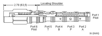
This valve is a 3-way, 3-position proportional directional valve. Port 3 is closed in the center position and port 2 and port 4 are drained to port 1. Pilot pressure at port 1 creates a metering orifice between ports 3 and 4 that is proportional to the pressure at 1. Piloting 6 opens 3 to 2. The force balance of the flow forces, spring and pilot pressure results in a degree of partial self-compensation as the load pressure changes.
