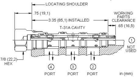
High accuracy, closed-center flow divider/combiners are sliding-spool, pressure-compensated devices used to split flow in one direction and combine flow in the opposite direction. These valves may be used to accurately control two or more cylinders or hydraulic motors where bidirectional operation is required.
