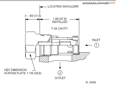
This valve was designed to be used in a parts-in-body, hot oil shuttle assembly. 2 valves, nose to nose, with a pin in between created the low side shuttle.
