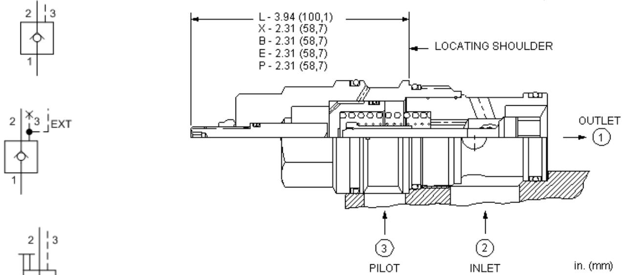
This valve is a pilot to open check valve. It has a sealed pilot, a steel seat, and is non-vented. It allows free flow from the valve (port 2) to the load (port 1) and blocks flow in the opposite direction. Pressure at the pilot (port 3) will open the valve from port 1 to port 2. Pilot pressure needed at port 3 to open the valve is directly proportional to the load pressure at port 1. Pressure at port 2 directly opposes pilot pressure.
