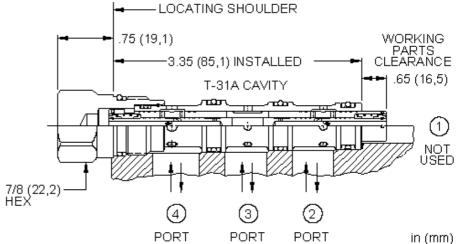
Synchronizing flow divider/combiners are sliding-spool, pressure-compensated devices used to split flow in one direction and combine flow in the opposite direction. With a sychronizing feature, these valves can be used to allow two hydraulic cylinders to fully stroke and synchronize at the end of the stroke. When the first cylinder has reached the end of its stroke, a pressure-compensated, reduced flow is metered to or from the second cylinder until it also reaches the end of its stroke.
