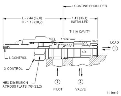
This valve is a pilot to open check valve. It has a sealed pilot, a steel seat, and is non-vented. It allows free flow from the valve (port 2) to the load (port 1) and blocks flow in the opposite direction. Pressure at the pilot (port 3) will open the valve from port 1 to port 2. Pilot pressure needed at port 3 to open the valve is directly proportional to the load pressure at port 1. Pressure at port 2 directly opposes pilot pressure.
