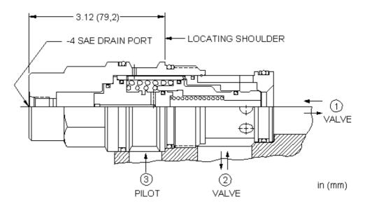
This is a normally closed, balanced poppet, switching element. When the external vent port is blocked, the poppet remains in the closed position. Venting the external port shifts it to the open position, provided there is sufficient pressure at port 3.
