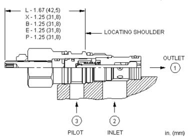
This valve is a pilot to open check valve. It has a sealed pilot, a steel seat, and is non-vented. It allows free flow from the valve (port 2) to the load (port 1) and blocks flow in the opposite direction. Pressure at the pilot (port 3) will open the valve from port 1 to port 2. Pilot pressure needed at port 3 to open the valve is directly proportional to the load pressure at port 1. Pressure at port 2 directly opposes pilot pressure.
