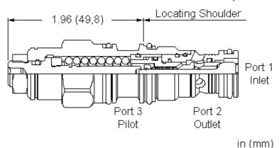
Counterbalance valves with pilot assist are meant to control an overrunning load. The check valve allows free flow from the directional valve (port 2) to the load (port 1) while a direct-acting, pilot-assisted relief valve controls flow from port 1 to port 2. Pilot assist at port 3 lowers the effective setting of the relief valve at a rate determined by the pilot ratio.
