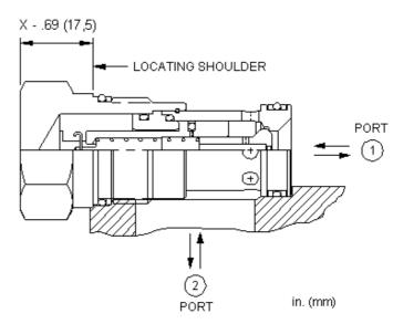
Air-bleed and start-up cartridges are used to purge air trapped in the system to help reduce power requirements and facilitate pump priming during the start-up of blocked center circuits.
