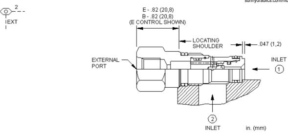
The single ball shuttle connects the higher of two work ports to the signal or common port. The signal is sensed at an external port located in the hex-end of the cartridge.
