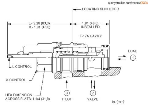
This valve is a pilot to open check valve. It has a non-sealed pilot, a Delrin seat, and is non-vented. It allows free flow from the valve (port 2) to the load (port 1) and blocks flow in the opposite direction. Pressure at the pilot (port 3) will open the valve, allowing flow from port 1 to port 2. Pilot pressure needed at port 3 to open the valve is directly proportional to the load pressure at port 1. Pressure at port 2 directly opposes pilot pressure.
