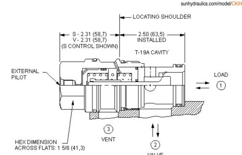
This valve is a pilot to open check valve. It has a non-sealed pilot, a steel seat, and is vented. It allows free flow from the valve (port 2) to the load (port 1) and blocks flow in the opposite direction. Pressure at the external pilot port will open the valve from port 1 to port 2. Pilot pressure needed to open the valve is directly proportional to the load pressure at port 1. The valve is insensitive to pressure at port 2 because the spring chamber references the vent (port 3).
