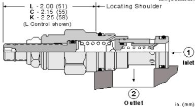
Kick-down relief cartridges act similar to a circuit breaker in an electrical system. The valves will kick completely open and remain open once the pressure at the inlet (port 1) exceeds the valve settling, creating an unrestricted flow path from port 1 to tank (port 2). The valve remains open as long as the pressure at port 1 exceeds the pressure at port 2. To reset the valve, flow from port 1 to port 2 must cease and pressure at port 2 must be equal to or greater than the pressure at port 1.
