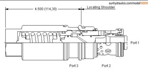
Balanced load control valves combine a balanced modulating element with a reverse flow check. The check valve allows free flow from the directional valve (port 2) to the load (port 1) while the pilot to open modulating element controls flow from port 1 to port 2. Pilot pressure at port 3 determines the flow setting.
