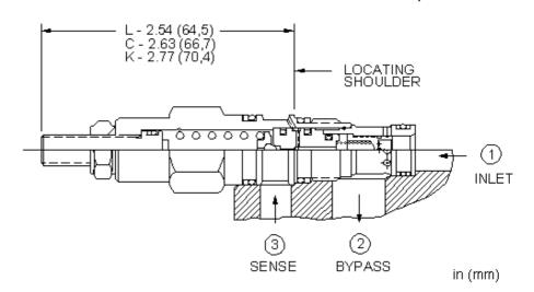
Three-port normally closed modulating elements with relief provide two functions when combined with an external orifice. The mainstage is a bypass compensator that controls a priority flow into the circuit, determined by the external orifice. Input flow in excess of the priority flow is bypassed to tank (port 2). If the inlet (port 1) pressure rises to the valve setting, the valve operates as a normal relief valve.
