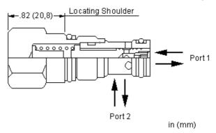
Flow fuse cartridges are used to maintain the position of a hydraulic actuator in the event of a hose or line break. The valve allows flow to and from the actuator but closes instantly if flow from the actuator exceeds the setting of the valve. NOTE: Because the valve responds so rapidly, it is sensitive to any transient flow above the valve setting.
