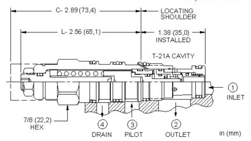
Vented counterbalance valves with pilot assist are meant to control an overrunning load. The check valve allows free flow from the directional valve (port 2) to the load (port 1) while a direct-acting, pilot-assisted relief valve controls flow from port 1 to port 2. Pilot assist at port 3 lowers the effective setting of the relief valve at a rate determined by the pilot ratio. Backpressure at port 2 does not affect the valve setting because the spring chamber references the vent (port 4).
