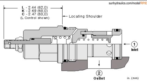
Fast-acting, pilot-operated, balanced piston relief cartridges are normally closed, pressure-limiting valves used to protect hydraulics components from pressure transients. Fast opening and closing is gained at the expense of smoothness. When the pressure at the inlet (port 1) reaches the valve setting, the valve starts to open to tank (port 2), throttling flow to limit the pressure rise. These valves have low pressure rise vs. flow and are very fast.
