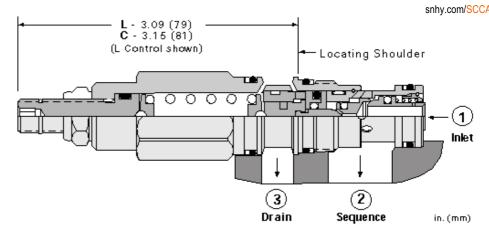
Direct-acting sequence valves with reverse-flow check will supply a secondary circuit with flow once the pressure at the inlet (port 1) has exceeded the valve setting. Additionally, these valves incorporate an integral check valve to provide reverse flow from port 2 (sequence) to port 1 (inlet). The pressure setting of a sequence valve controls the pressure at port 1 relative to the pressure at the drain (port 3).
