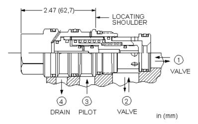
This is a normally open, balanced poppet, switching element. When the vent port (port 4) is blocked, the poppet remains in the open position. Venting port 4 shifts it to the closed position, provided there is sufficient pressure at port 3.
