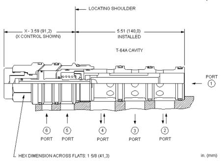
Two-position, detented, 4-way directional cartridges are 6-port directional valves that can be configured with up to 3 different spool options. The supply port is port 1 and all ports will accept 5000 psi (350 bar). Capacity for these pilotto-shift valves is dependent on the spool type specified.
