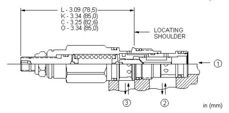
Direct-acting, 3-way directional cartridges (1 blocked, 2 to 3 open) are switching devices typically used in moderate flow circuits. They can be used by themselves or to actuate larger pilot-operated directional cartridges or logic cartridges. The valve shifts when the pressure differential between port 1 and port 3 exceeds the setting.
