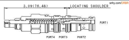
Direct-acting, 3-way directional cartridges (3 to 4 open, 2 blocked) are switching devices typically used in moderate flow circuits. They can be used by themselves or to actuate larger pilot operated directional cartridges or logic cartridges. The valve shifts when the pressure differential between port 1 and port 4 exceeds the setting.
