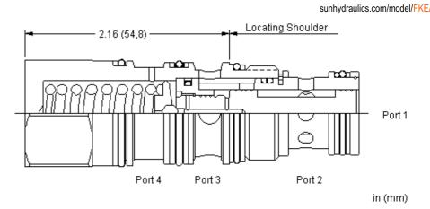
This valve is a 2-way, 2-position proportional throttle. Ports 2 and 3 are normally closed. Pilot pressure at port 1 creates a metering orifice between port 2 and 3 that is proportional to the pressure at 1. The force balance of the flow forces, spring and pilot pressure results in a degree of partial self-compensation as the load pressure changes.
