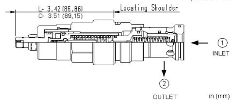
Pilot-operated, anti shock relief cartridges limit maximum system pressure and also limit the rate of pressure rise. The valve opens and then ramps closed at a constant speed, independent of settings and flows. The adjust screw determines the maximum (relief) setting and the minimum (threshold) setting.
