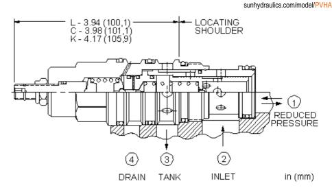
Externally drained, pilot-operated pressure reducing/relieving valves reduce a high primary pressure at the inlet (port 2) to a constant reduced pressure at port 1, with a full-flow relief function from port 1 to tank (port 3). Draining the pilot section at port 4 makes these valves insensitive to pressure at tank (port 3) and provides a means for remote control by pilot or 2-way valves.
