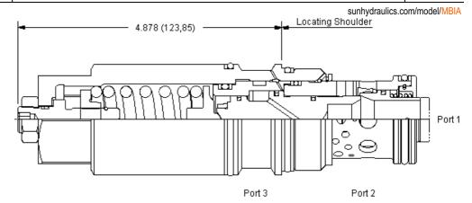
Load reactive, load control valves with pilot assist combine two valves; a check valve and a relief valve. The check valve allows free flow from the directional valve (port 2) to the load (port 1) while a direct-acting, pilot-assisted relief valve controls flow from port 1 to port 2. Pilot assist at port 3 lowers the effective setting of the relief valve at a rate determined by the pilot ratio.
