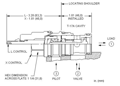
This valve is a pilot to open check valve. It has a sealed pilot, a Delrin seat, and is non-vented. It allows free flow from the valve (port 2) to the load (port 1) and blocks flow in the opposite direction. Pressure at the pilot (port 3) will open the valve from port 1 to port 2. Pilot pressure needed at port 3 to open the valve is directly proportional to the load pressure at port 1. Pressure at port 2 directly opposes pilot pressure.
