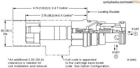
This solenoid controlled, 2-way, 2-position cartridge is a pilot-operated, poppet style directional valve with reverse free flow check. It is available in either a normally open or normally closed configuration. Due to its poppet style construction, it has extremely low leakage.
