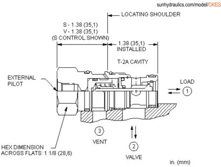
This valve is a pilot to open check valve. It has a non-sealed pilot, a Delrin seat, and is vented. It allows free flow from the valve (port 2) to the load (port 1) and blocks flow in the opposite direction. Pressure at the external pilot port will open the valve from port 1 to port 2. Pilot pressure needed to open the valve is directly proportional to the load pressure at port 1. The valve is insensitive to pressure at port 2 because the spring chamber references the vent (port 3).
