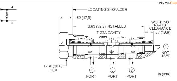
Synchronizing flow divider/combiners are sliding-spool, pressure-compensated devices used to split flow in one direction and combine flow in the opposite direction. With a sychronizing feature, these valves can be used to allow two hydraulic cylinders to fully stroke and synchronize at the end of the stroke. When the first cylinder has reached the end of its stroke, a pressure-compensated, reduced flow is metered to or from the second cylinder until it also reaches the end of its stroke.
