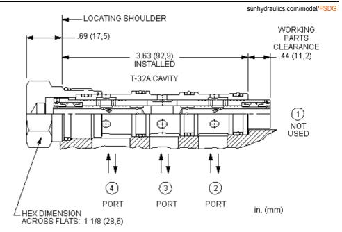
High accuracy, closed-center flow divider/combiners are sliding-spool, pressure-compensated devices used to split flow in one direction and combine flow in the opposite direction. These valves may be used to accurately control two or more cylinders or hydraulic motors where bidirectional operation is required.
