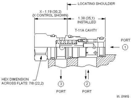
Direct-acting, 3-way directional cartridges (1 blocked, 2 to 3 open) are switching devices typically used in moderate flow circuits. They can be used by themselves or to actuate larger pilot-operated directional cartridges or logic cartridges. The valve shifts when the pressure differential between port 1 and port 3 exceeds the setting.
