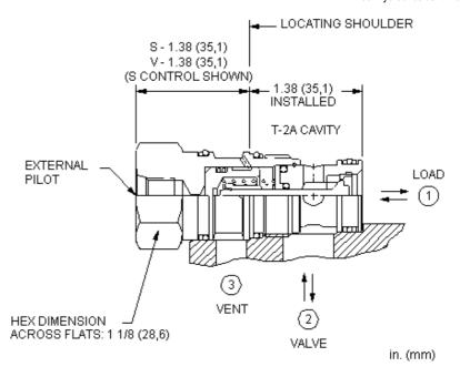
This valve is a pilot to open check valve. It has a non-sealed pilot, a steel seat, and is vented. It allows free flow from the valve (port 2) to the load (port 1) and blocks flow in the opposite direction. Pressure at the external pilot port will open the valve from port 1 to port 2. Pilot pressure needed to open the valve is directly proportional to the load pressure at port 1. The valve is insensitive to pressure at port 2 because the spring chamber references the vent (port 3).
