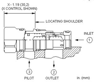
This valve is a spring biased closed, pilot-to-close check cartridge that has a 1.8:1 pilot ratio. The valve allows flow from port 1 to port 2 and blocks reverse flow. Pressure at the pilot port opposes pressure at port 1 at a ratio of 1.8:1. This valve is most often used in regeneration circuits.
