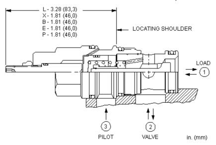
This valve is a pilot to open check valve. It has a non-sealed pilot, a steel seat, and is non-vented. It allows free flow from the valve (port 2) to the load (port 1) and blocks flow in the opposite direction. Pressure at the pilot (port 3) will open the valve from port 1 to port 2. Pilot pressure needed at port 3 to open the valve is directly proportional to the load pressure at port 1. Pressure at port 2 directly opposes pilot pressure.
