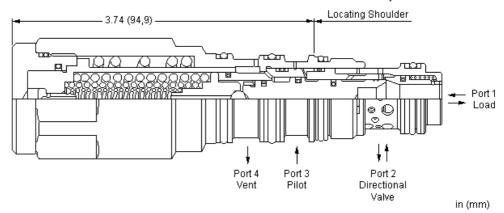
These valves are self-setting counterbalance valves which combine multiple functions in one package; reverse free flow, load, and thermal relief. The check allows free flow from the directional valve (port 2) to the load (port 1) while a direct-acting pilot function self adjusts to approximately 1.3 times the load induced pressure up to the thermal relief setting. Backpressure at port 2 does not affect self setting performance because the spring chamber references the vent (port 4).
