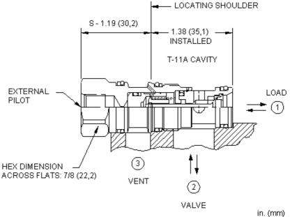
This valve is a pilot to open check valve. It has a sealed pilot, a Delrin seat, and is vented. It allows free flow from the valve (port 2) to the load (port 1) and blocks flow in the opposite direction. Pressure at the external pilot port will open the valve from port 1 to port 2. Pilot pressure needed to open the valve is directly proportional to the load pressure at port 1. The valve is insensitive to pressure at port 2 because the spring chamber references the vent (port 3).
