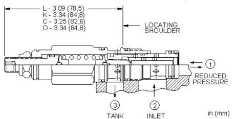
Direct-acting, pressure reducing valves reduce a high primary pressure at the inlet (port 2) to a constant reduced pressure at port 1. These valves incorporate a damped construction for stable operation allowing the use of high reduced pressure. This valve is open in the transition from reducing to relieving. It provides good pressure control and dynamic response.
