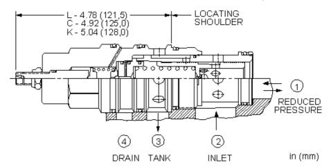
Externally drained, pilot-operated pressure reducing/relieving valves reduce a high primary pressure at the inlet (port 2) to a constant reduced pressure at port 1, with a full-flow relief function from port 1 to tank (port 3). Draining the pilot section at port 4 makes these valves insensitive to pressure at tank (port 3) and provides a means for remote control by pilot or 2-way valves.
