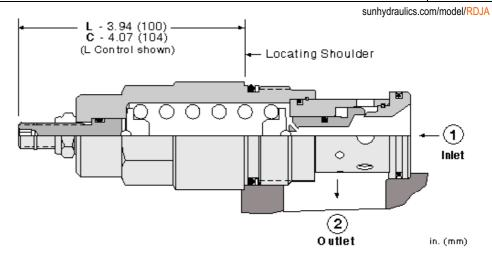
Direct-acting relief cartridges are normally closed, pressure-limiting valves used to protect hydraulic components from pressure transients. When the pressure at the inlet (port 1) reaches the valve setting, the valve starts to open to tank (port 2), throttling flow to limit the pressure rise. These valves are smooth and quiet, essentially zero leak, dirt tolerant, immune to silting and are very fast.
