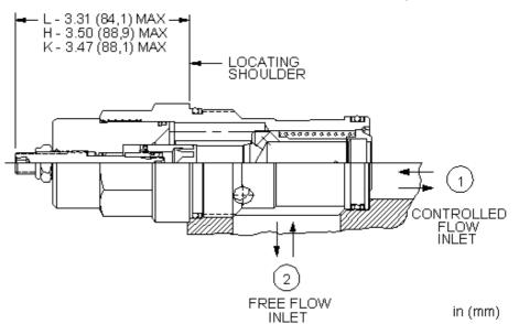
Needle valves with reverse-flow check are fully adjustable orifices used to regulate flow. They are infinitely adjustable from fully closed up to the maximum orifice diameter. An integral high-capacity check valve provides unrestricted flow from port 2 to port 1. They are not pressure compensated.
