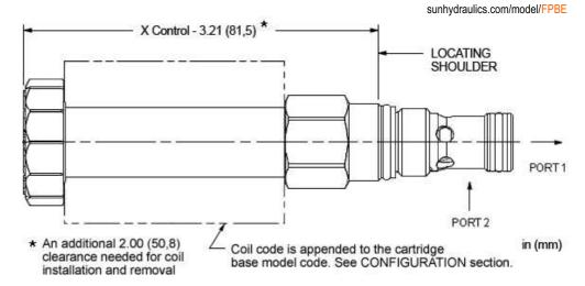
This valve is a pilot-operated, normally closed, electro-proportional throttle with reverse free-flow check. Energizing the coil generates an opening force on the pilot stage which vents the main stage poppet to open proportionally, allowing flow from port 2 to 1. The check will allow flow from 1 to 2 in either the open or closed condition.
