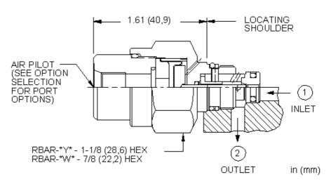
Two-port, pilot-stage, air-controlled, direct-acting relief cartridges are normally closed pressure regulating valves. When the pressure at port 1 (inlet) is sufficient to overcome the force due to the air signal, a flow path is opened from port 1 to port 2 (tank). These cartridges are designed for pilot flow applications and utilize Sun's T-8A cavity so they can be used in conjunction with Sun's pilot-operated, main-stage valves.
