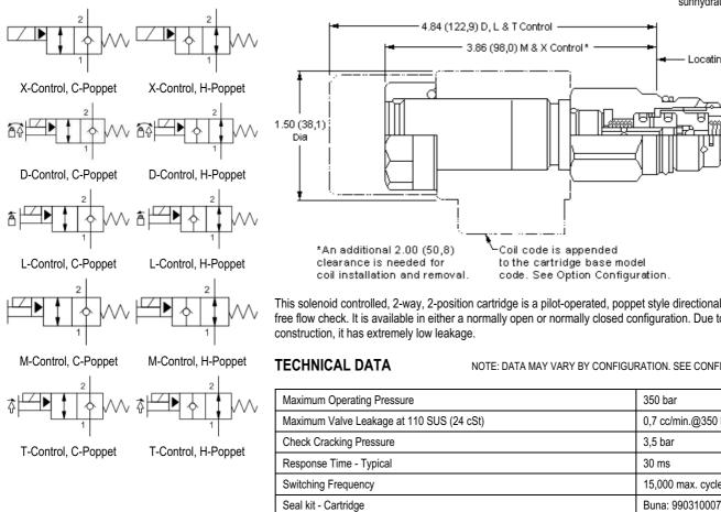
· Please verify cartridge clearance requirements when choosing a Sun manifold. Different valve controls and coils require different clearances. NOTES
