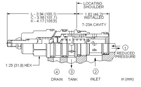
Externally drained, pilot-operated pressure reducing/relieving valves reduce a high primary pressure at the inlet (port 2) to a constant reduced pressure at port 1, with a full-flow relief function from port 1 to tank (port 3). Draining the pilot section at port 4 makes these valves insensitive to pressure at tank (port 3) and provides a means for remote control by pilot or 2-way valves.
