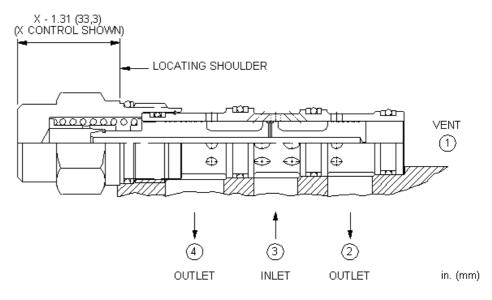
This vent-to-shift diverter valve is a 2-position, 3-way cartridge that is normally open from port 3 to port 4. When port 1 is vented, the pressure differential between port 3 and port 1 exceeds the spring force causing the valve to shift, thereby connecting port 3 to port 2.
