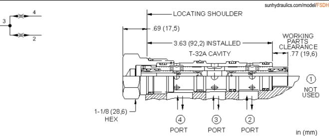
High-capacity, closed-center flow divider/combiners are sliding-spool, pressure-compensated devices used to split flow in one direction and combine flow in the opposite direction. These valves have approximate 15% greater capacity than standard closed-center divider/combiners and are designed for use in tractive drive systems. Note: Accuracy on these cartridges is not equivalent to the accuracy of standard closed-center divider/combiners.
