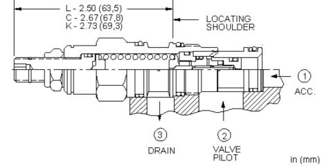
The accumulator sense, pump unload pilot valve is used to sense pressure in an accumulator at port 1 of the valve and when the pressure at port 1 reaches the valve setting, port 2 connects to port 3 to vent a relief valve and unload the pump. This valve has a 20% ratio between unload setting and reset; when pressure at port 1 falls below 80% of the valve setting, port 2 is blocked from port 3 and the pump will come back online to recharge the accumulator.
